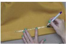
**32.** Center and line the LED strip along the bottom edge of the hem and mark where the LED strip's end is.
