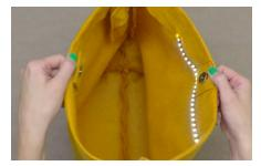
**51.** The lights will turn on when the bag is opened and the magnet moves away from the switch.
