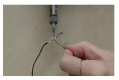
**15.** Solder the other end of the 18" hookup wire to the normally closed pin on the reed switch.
