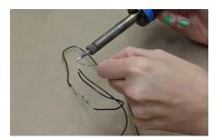
**18.** Solder the ground wire of the battery clip to the 5" hookup wire that is attached to the reed switch.
