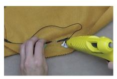
**43.** Glue one of the taped connections on the switch, not the switch itself, to the back of the purse clasp.
