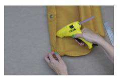
**45.** Make sure all wires except for the battery clip's are tucked under the hem. Glue the hem down.
