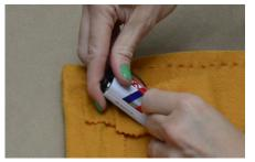
**48.** Snap the clip onto the battery and tuck it into the pouch.
