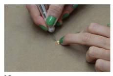
**10.** Prepare the LED strip by lightly scraping the positive and ground connections with a craft knife.
