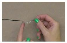
**14.** Test your reed switch to find out which pin is "normally closed". When attached to a battery and an LED, the LED should be off when a magnet is near the switch.
