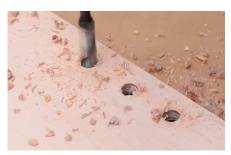
**21.** Drill some holes through the back of the electronic components side of your tray. This is where the wires will go.
