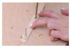
**9.** Drill a 1/4" hole into the launcher where you made the mark in step 8.
