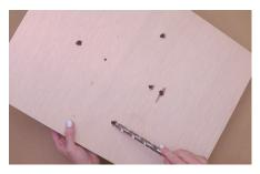
**20.** Use the 5/8" drill bit at an angle to "tune" the five ball holes on the back of the board. Make them slant downwards so that the pachinko balls can easily roll out.
