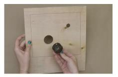
**21.** Find a piece of plywood large enough to hold the lamp that you want to design. Ours is 10" x 11". Drill a hole large enough for the lamp socket to fit through.
