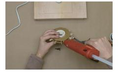
**33.** Next apply hot glue to the corrugated space on your large gear and wedge the other side of your hookup wire angle in between the layers of corrugation.
