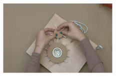
**25.** Mount your smaller gear so that the dowels will hit the craft sticks directly in the middle of each stick. Glue the motor in place once you have found the correct height it should be at.
