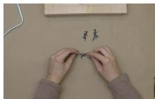
**32.** To attach your design, cut and strip some hookup wire and bend it at a right angle. Glue one side of the angle to your cutout.
