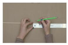
**15.** Measure and cut five 1.5" long pieces from the wooden dowel. Sand the edges down.
