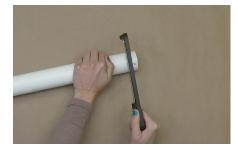
**4.** Measure and mark one inch of PVC pipe. Cut it off with the hack saw. Sand the sawed edges down.
