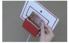
**39.** Using the copper tape, attach one hookup wire to the copper side of the index card and the other hookup wire to the copper on the bottom of the basket
