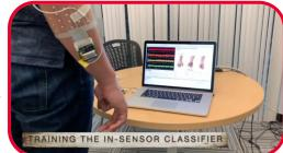
to your hand muscles to do that task. As the signals travel through neurons in your arm, the device can detect the patterns and mimic the motion on a screen or with a robotic arm. This technology could be used to help people with limb loss better control a prosthetic or to interact inside a video game. Another new advance that relies on electronics and circuitry is artificial skin for robots. As robots are taking on more tasks, and sometimes working alongside humans, it's important
